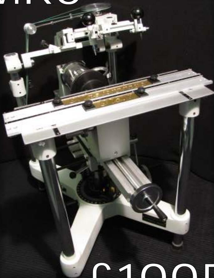
The MK-5 Universal Engraving Machine is probably the most versatile engraving machine in the world. It is capable of engraving both flat and bulky / cylindrical items, using the same vice assembly.
