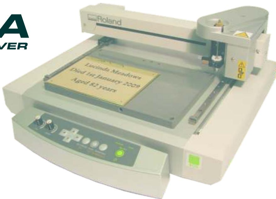
The EGX-30A makes engraving easy. Simply use the software to design your badge, nameplate or plaque and generate the engraving path. Then, with a push of a button, the desktop device automatically detects the material's thickness when the tip of the nose guard touches the surface. While engraving, you can effortlessly adjust the feed rate and spindle rpm by simply turning the knob located on the control panel.
