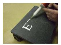
When character is filled, remove finger from trigger to stop flow.
