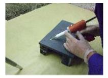
Put nozzle into 1st character to be filled and pull trigger slowly to allow paint to flow.
