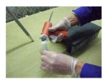
Fit barrel to gun by pushing it hard over the rubber seal/"O" ring and twist anti clockwise to lock into place on the gun flange.
